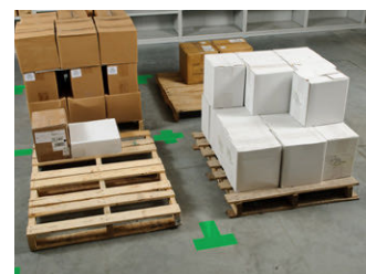
3. Colour-code material storage areas.
